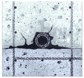
Honey-combs and cracks will be filled with injection resin completely. This will produce a watertight concrete structure. Injection-402 is available prefabricated or as kit. The prefabricated hoses consists from 10 m injection hose and two 70 cm vent ends in different colors. Packaging is 5 pcs. in a cardboard (=50 m)
