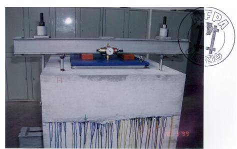
With HydroBloc Injekt 583 injected reinjectable hose
