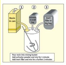
Pour the resin into a clean plastic or other suitable container and gradually add the small bag containing hardener. Mix thoroughly. Now add the large bag containing filler and mix until a uniform colour and consistency is achieved.
